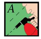
A im low and direct the extinguisher at the base of the fire.
