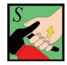
S queeze the handle slowly and evenly. Continue to squeeze until the fire is out and/or the fire extinguisher is empty.
